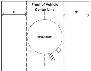
The distance from the edge of the roof to the rear corner of the foot should be equal on both sides of the dish to ensure proper installation.
